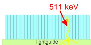
Fig. 2: The scintillation light caused by a gamma particle is spatially confined in a pixelated detector.
