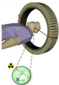
Fig. 1: In PET, two 511 keV gamma photons from a positron-electron annihilation have to be detected and correlated.
