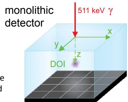
Fig. 3: A cuboid, monolithic detector block concept. (reprinted from Van Dam, H. T. et al. (2011). “A practical method for depth of interaction determination in monolithic scintillator PET detectors”. Phys. Med. Biol., 56(13), 4135–4145. doi:10.1088/0031-9155/56/13/025)
