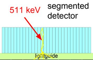
Fig. 2: The scintillation light caused by a gamma particle is spatially confined in a pixelated detector. The scintillator segments are isolated from each other by reflective foils.
